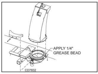
Figure 12. Chute Base and Rotator Ring
